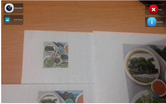
Fig. 19. Application can not detect marker 15% smaller.
